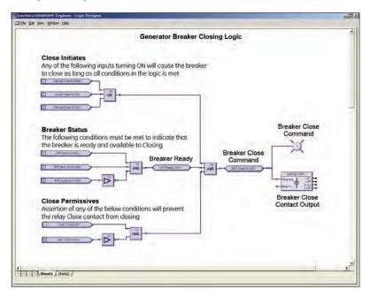
Flexlogic allows for customizing the G30 to operate and control the breakers and other auxiliary devices needed to fit most generator protection schemes and applications.
