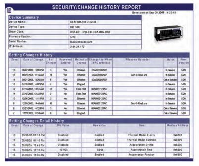
The G30 tracks and records information about configuration changes that have been made to the relay thereby providing a method of auditing system security and engineering processes
