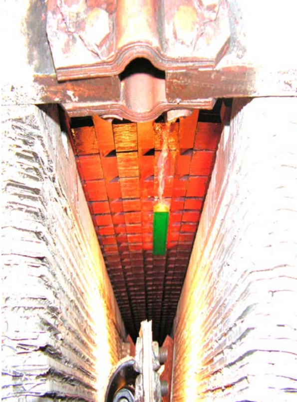
Fig. 12 Air gap Sensor on the stator wall
